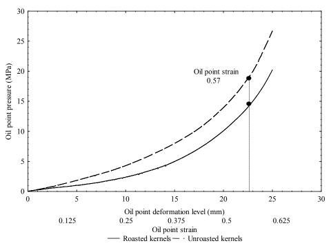
**Fig. 2.** Oil point pressure versus deformation level and strain of bulk roasted and unroasted kernels at pressing height 40 mm and speed 5 mm min<sup>-1</sup>.
